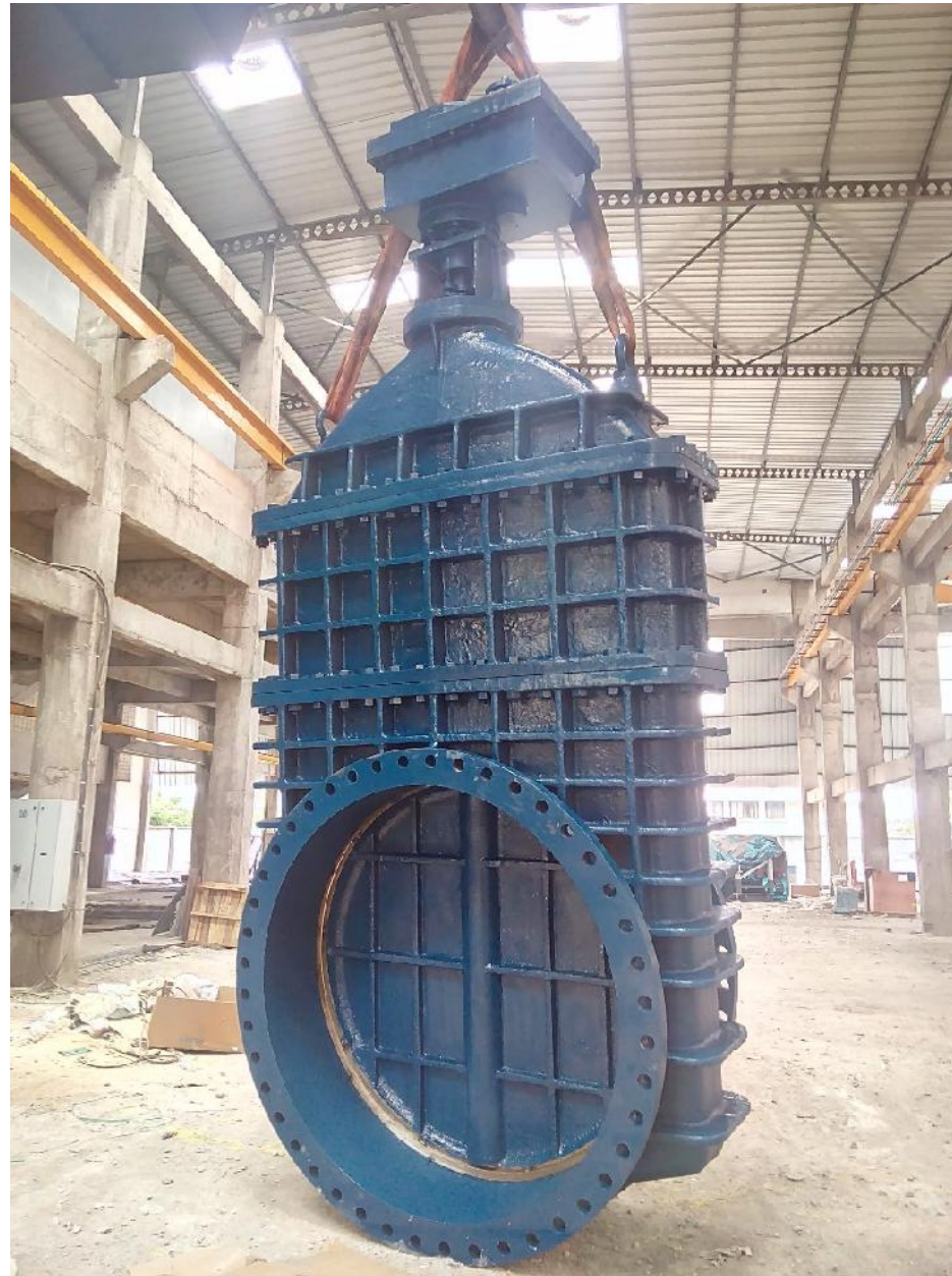
This is a photo of the largest sized (1800mm) metal-seated gate valve to have been built in India till date, ready to be shipped from our works in Pardi, Gujarat
